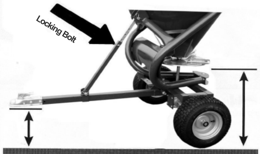
Correct position of the spreading disc.
